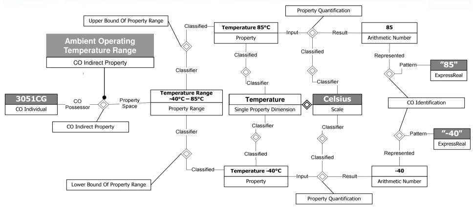
3051CG has a "ambient operating temperature": -40 C-85 C
