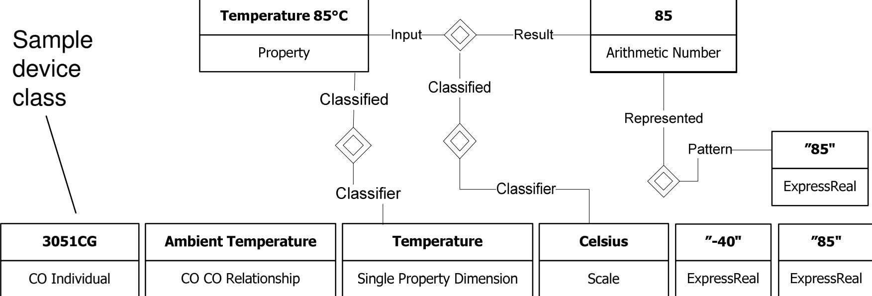
“The ambient temperature during operation of a 3051CG pressure transmitter should be within -40 and 85 degrees Celsius.”
