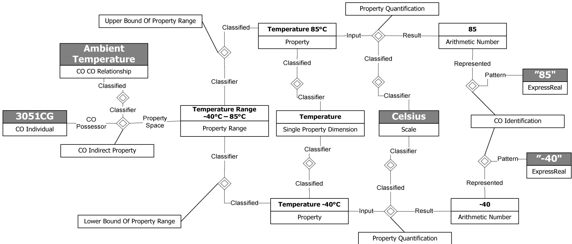
3051CG ambient temperature:  $-40^{\circ}\text{C} - 85^{\circ}\text{C}$
