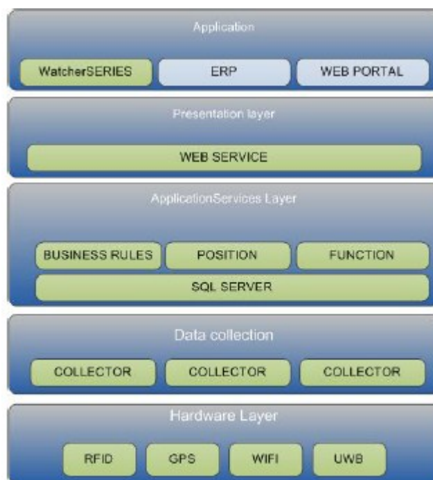
Figure 3.10 An example RDID application stack
