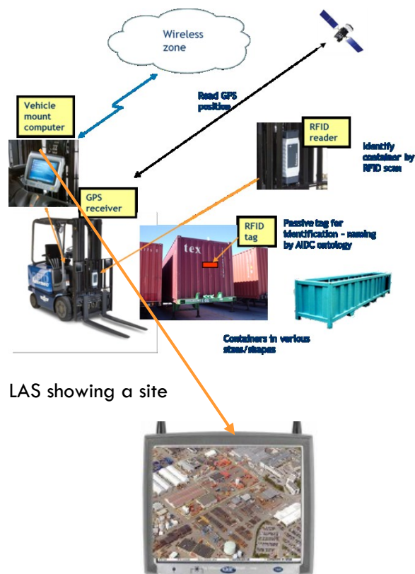
Figure 3.7 Tracking equipment on the forklift truck including LAS
