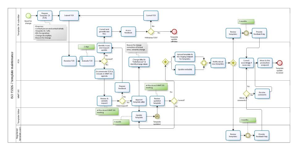
Figure 2. Process to update an existing template
