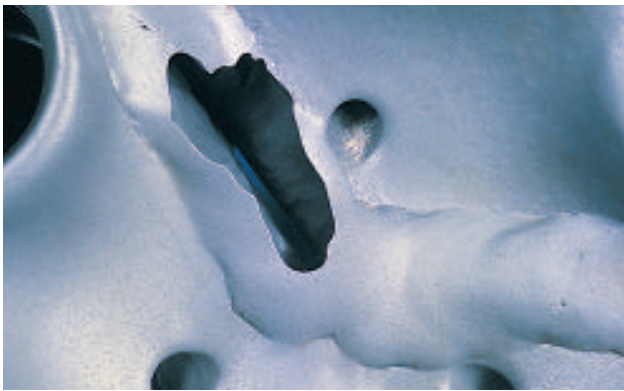
WELD WASH OUT (WO)
