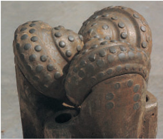
GRADED DULL NO. 2 (5, 8, WT, A, 3, 2, FC, HRS)
