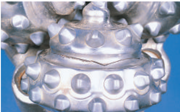
CRACKED CONE (CC)
