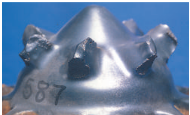
SELD-SHARPENING WEAR (SS)
