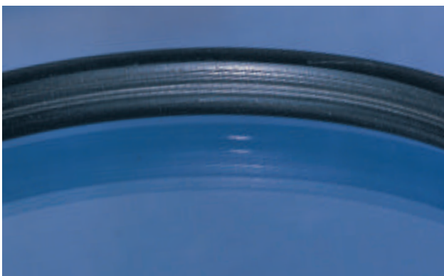
WORN SEAL (Denoted as SF)
