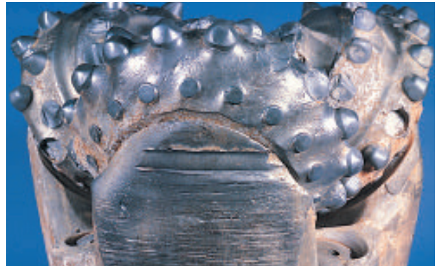
JUNK DAMAGE (JD)
